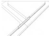
Spanners are used to provide a bridge between panels for the Thinglow Lighting. Spanners are installed after the panels have been mounted. Each spanner comes with two adhesive pieces at each end. Remove the protective plastic, and adhere it to the one inch high white vertical surface on the panels light cove.
